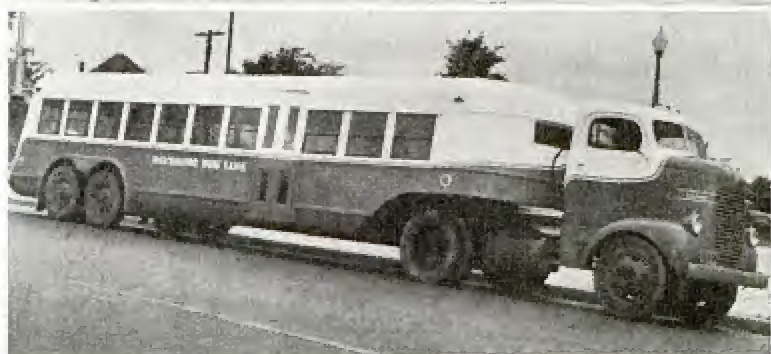
Bus, bottom, was converted from an auto transport trailer like the one above, opening a useful life for trailer that had lost its regular job
